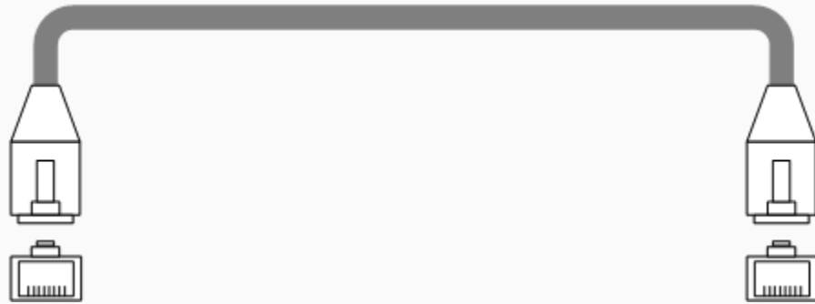
Figure 4 – Cable for Ethernet Connection
